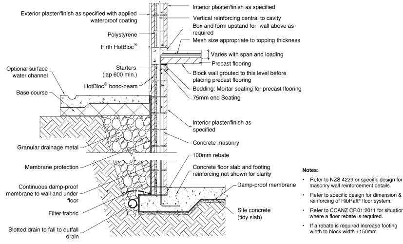
Note: refer to NZS 4229 or specific design for masonry reinforcing
